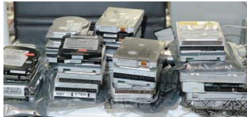
A typical sight in Dr. Payne's basement — stacks of used hard drives await testing and formatting before they can be installed into newly rebuilt computers.
